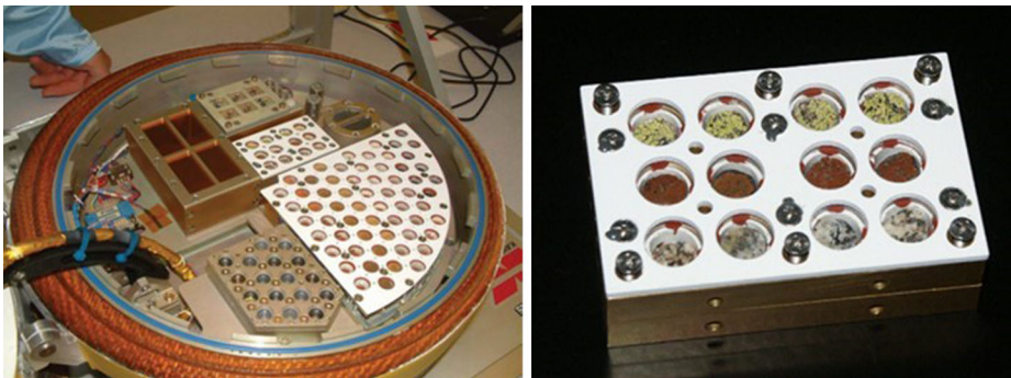
Fig. 35 On the left picture Biopan-5 when it was opened immediately after the flight, including the LICHENS experiments, shown in details in the picture on the right . Arrow shows the position of the experiment LICHEN
