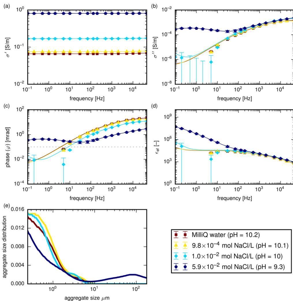
**Fig. 9.** In-phase conductivity (a), quadrature conductivity (b), phase (c), effective dielectric permittivity (d) as a function of frequency, and computed aggregate size distributions (e) of 1.5% Na-Mt dispersions at different added NaCl concentrations. Symbols are experimental data and lines are calculations from the complex conductivity model.
