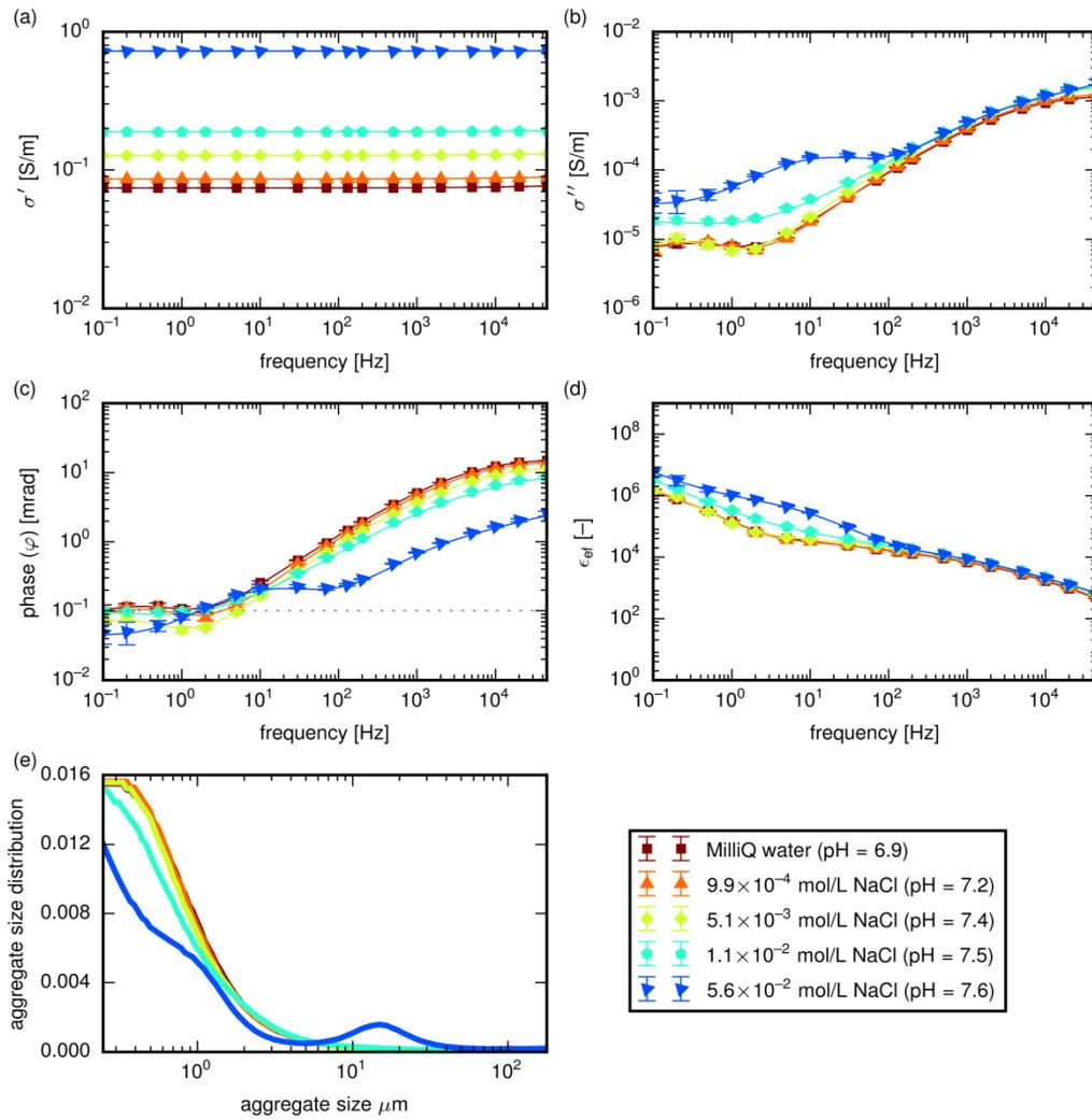
**Fig. 10.** In-phase conductivity (a), quadrature conductivity (b), phase (c), effective dielectric permittivity (d) as a function of frequency, and computed aggregate size distributions (e) of 1% Na-Mt dispersion at pH = 7.3 and at different added NaCl concentrations. Symbols are experimental data and lines are calculations from the complex conductivity model.
