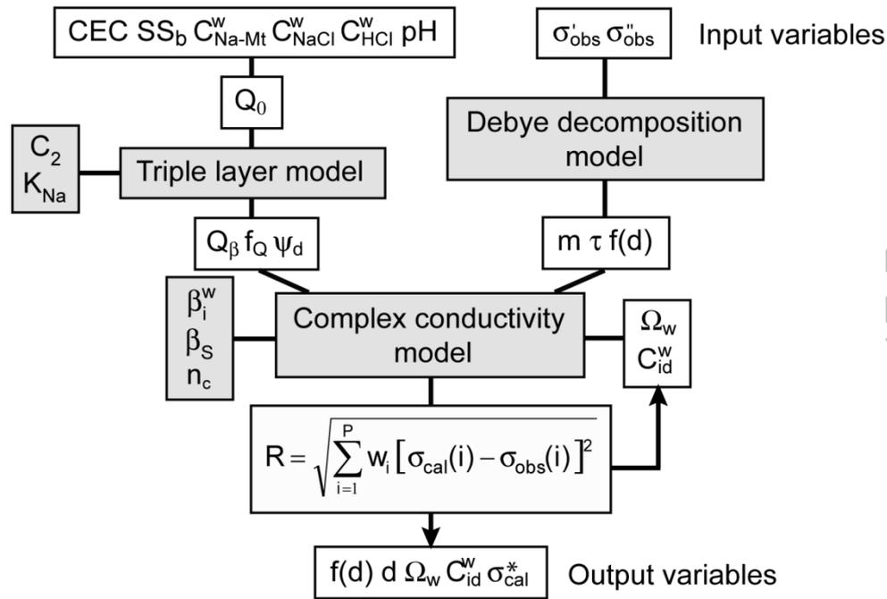
**Fig. 6.** Sketch summarizing the modeling strategy used to interpret complex conductivity spectra of Na-Mt dispersions (the inversion procedure used by the DD approach is not explained here, for more details, read Ref. [76]).
