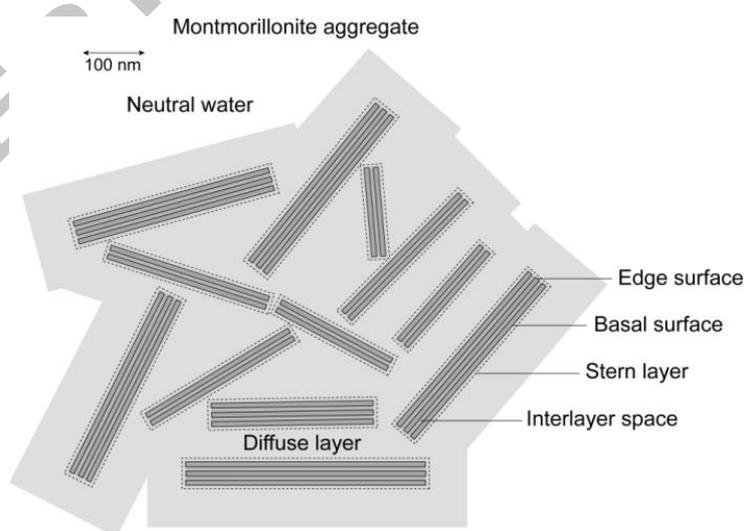
**Fig. 2.** Sketch of a Mt aggregate containing Mt particles surrounded by their Stern and diffuse layer (the thickness of the particles is larger than in reality, from Ref. [16] with the permission of the Publisher).
