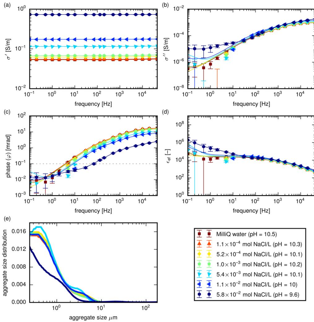
**Fig. 8.** In-phase conductivity (a), quadrature conductivity (b), phase (c), effective dielectric permittivity (d) as a function of frequency, and computed aggregate size distributions (e) of 1% Na-Mt dispersions at different added NaCl concentrations. Symbols are experimental data and lines are calculations from the complex conductivity model.
