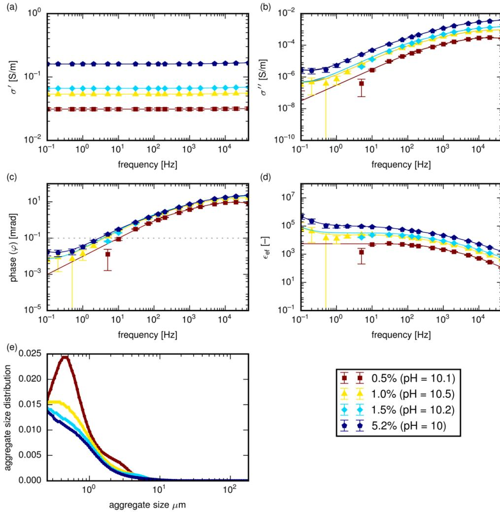
**Fig. 7.** In-phase conductivity (a), quadrature conductivity (b), phase (c), effective dielectric permittivity (d) as a function of frequency, and computed aggregate size distributions (e) of Na-Mt dispersions of weight fractions 0.5, 1, 1.5, and 5.2%. Symbols are experimental data and lines are the calculations from the complex conductivity model.
