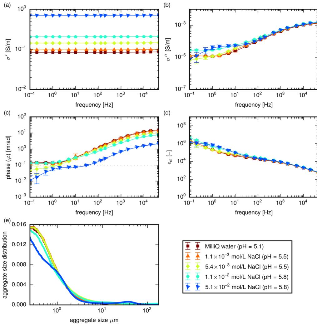
**Fig. 11.** In-phase conductivity (a), quadrature conductivity (b), phase (c), effective dielectric permittivity (d) as a function of frequency, and computed aggregate size distributions (e) of 1% Na-Mt dispersion at pH = 5.5 and at different added salinities (NaCl). Symbols are experimental data and lines are calculations from the complex conductivity model.
