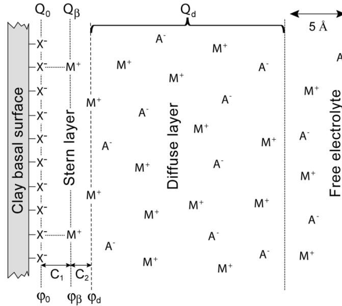
**Fig. 3.** TLM of the basal surface of Na-Mt in contact with a 1:1 electrolyte (e.g., NaCl). The parameters “ $\phi$ ”, “ $Q$ ” and “ $C$ ” stand for the electrical potential, the surface charge density, and the capacitance, respectively (from Ref. [16] with the permission of the Publisher).
