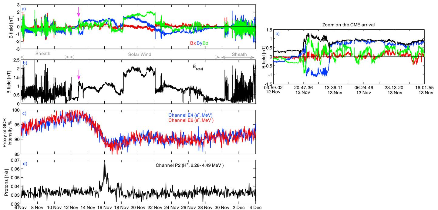
**Figure 8.** Observations of the shock and ICME arrival at Saturn by the Cassini spacecraft. (a and b) Components and magnitude of the magnetic field, respectively. (c) Proxy for the GCR, obtained from the E4 and E6 channels of the LEMMS sensor. (d) LEMMS proton channel with energy 2.4–4.2 MeV. (e) Zoom on the magnetic field data (Figures 8a and 8b together) to facilitate the identification of the arrival time of the ICME at Saturn (Table 1).
