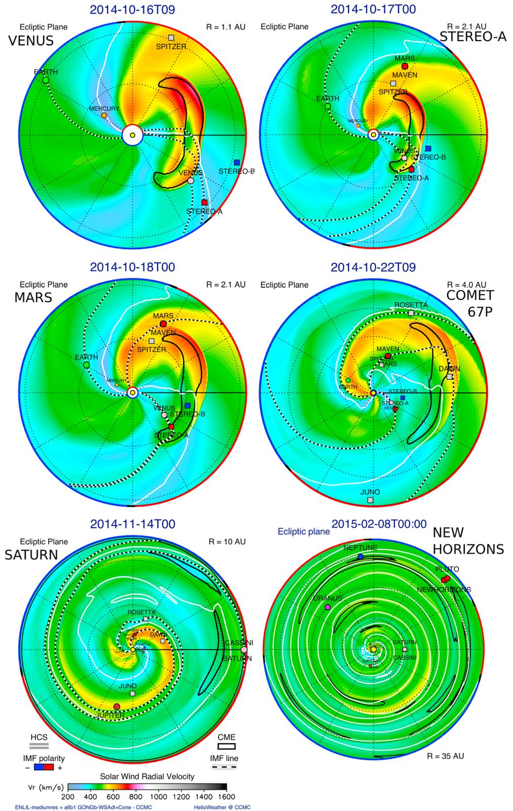
**Figure 3.** Stills of the solar wind velocity in the ecliptic plane from a WSA-ENLIL + Cone model simulation showing the ICME propagation, selected at the times of ICME closest approach to Venus, STEREO-A, Mars, comet 67P, Saturn, and New Horizons. The full simulations are available at <http://ccmc.gsfc.nasa.gov>; run numbers Leila\_Mays\_092716\_SH\_1 and Leila\_Mays\_100116\_SH\_1. The colors represent the speed, as indicated in the color scale.
