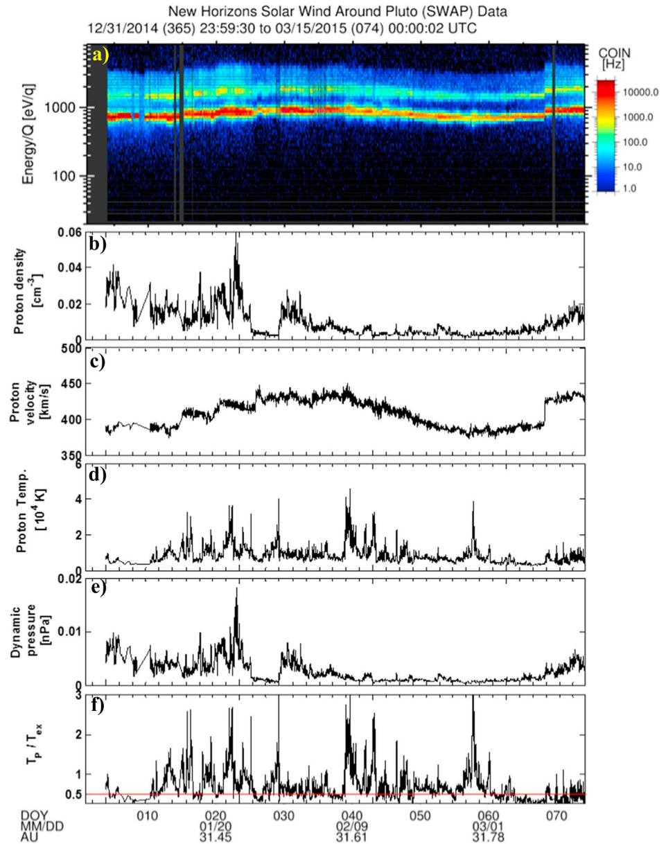
**Figure 9.** New Horizons SWAP data. (a) Ion spectrogram, with the top and bottom traces representing alpha particles and protons, respectively. (b–f) Solar wind density, speed, temperature, dynamic pressure, and ratio between the proton temperature and the expected temperature, as a possible ICME indicator [Elliott et al., 2012]. When that ratio is below 0.5, the interval could be an ICME. The period covers the first 80 days of 2015.
