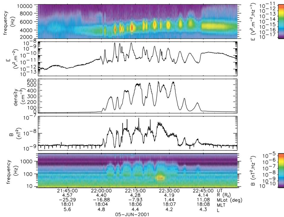
**Figure 2.** Correlation between whistler mode waves and density. From top to bottom, the panels show the (a) WHISPER electric field spectrogram below 10 kHz, (b) WHISPER frequency integrated electric intensity, (c) WHISPER-EFW density estimate, (d) STAFF frequency integrated magnetic intensity, (e) STAFF magnetic field spectrogram.
