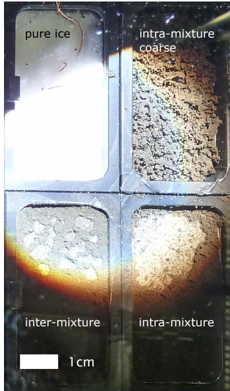
Figure 7: Experiment #3 during the 2nd illumination cycle. It is obvious that the residue layer is only ejected inside the illuminated areas, the shape of the intra-mixture patch follows exactly the spot geometry. The intra-mixture (lower left sample) residue layer is more cohesive than the one from the inter-mixture. The coarse fraction of intra-mixture shows no structural dichotomy between the illuminated and shadowed areas.
