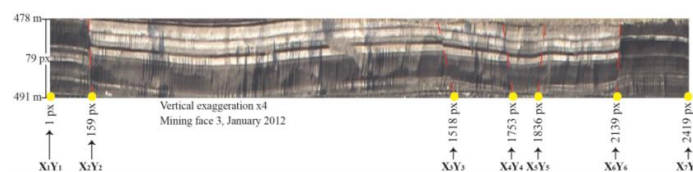
Figure 5 – An example of part of a mine face cropped from a panoramic photograph, showing the data required in order to import it into TrapTester. The X_iY_i coordinates and the corresponding pixels of the faults and the left and right end of the picture are needed to create the navigation lines. The X_iY_i coordinates for the left and right end of the picture are not known but they can easily be calculated as the number of pixels per meter is known. The altitude at the bottom of the picture is known and again using the pixels per meter, the altitude at the top can be calculated.
