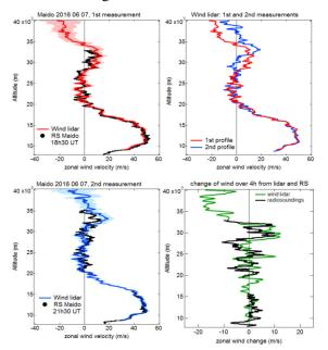
Figure 3. Verification of lidar temporally-resolved wind measurements using two radiosoundings: (top and bottom left) comparison of radiosonde and lidar wind profiles for the two consecutive soundings; (top right) comparison of two independent lidar profiles separated in time by 3 h; (bottom right) wind change over 3 h observed by lidar and radiosondes.
