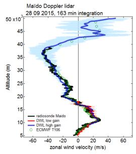
Figure 1. Comparison of zonal wind profiles obtained using Maido Doppler wind lidar on 28.09.2015 with collocated radiosounding and ECMWF operational analysis. Shaded areas indicate the total error of lidar retrieval.
