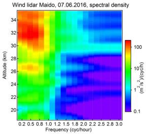
Figure 4. Power spectrum of stratospheric gravity wave frequency as a function of height derived from Maido wind lidar acquisition on 07.06.2016
