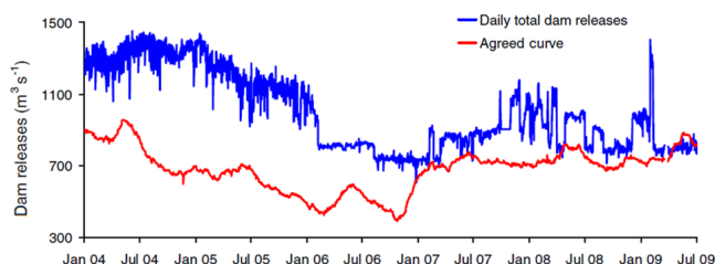
Figure 2. Observed daily total dam releases (blue line) and the agreed curve (red line) at the outlet of Lake Victoria in Jinja from November 2007 to July 2009 (Owor et al., 2011).
