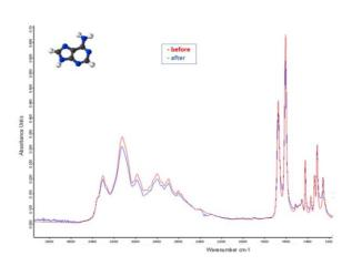
Figure 1: IR spectrum of a thin film of adenine before (in red) and after (in blue) being exposed on the International Space Station.
