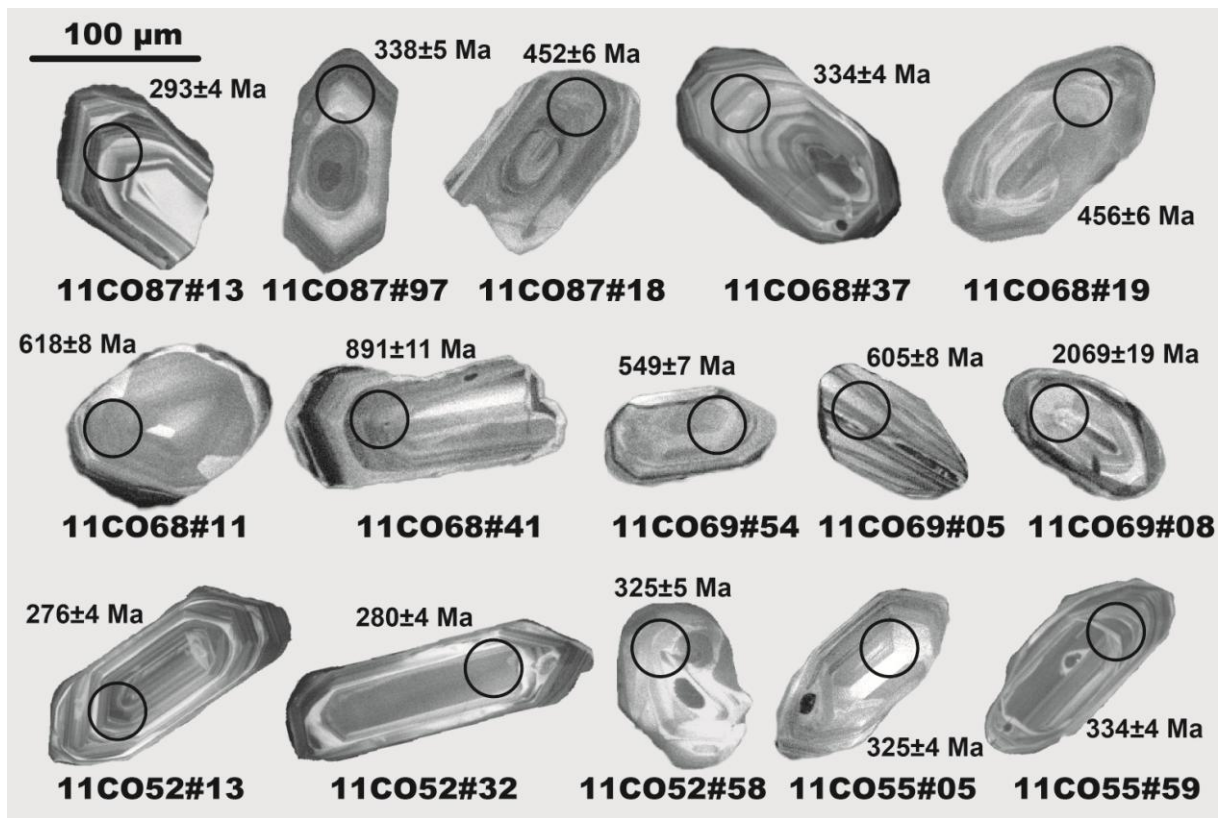
Fig. 7. Representative cathodoluminescence (CL) images of selected detrital zircons with a wide range in size and morphology from the Alpine turbidites of Corsica. The circles represent U-Pb analytical sites, numbers and ages presented in figure 8.
