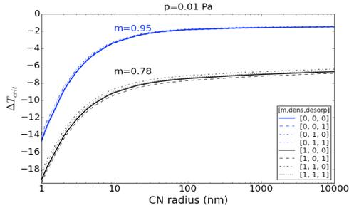
Figure 2: The temperature deviation required for IN activation as a function of the IN radius. The atmospheric pressure is 0.01 Pa (75 km). The blue lines show the results for contact parameter  $m=0.95$  and the black lines for  $m=0.78$ . The legend shows the variation of the different parameters: 0=old value, 1=new value.
