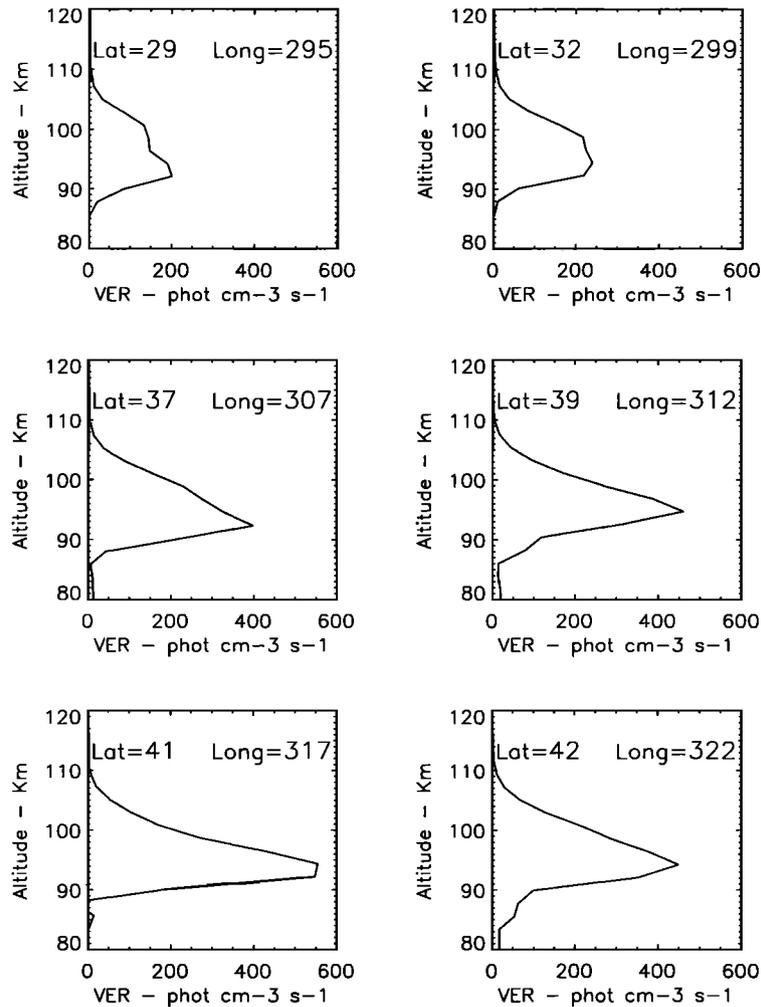
**Figure 9a.** A sequence of volume emission rate profiles taken by WINDII along the spacecraft track on March 31 near a longitude of  $300^{\circ}$ . The latitude, longitude, and local time for each profile are shown.
