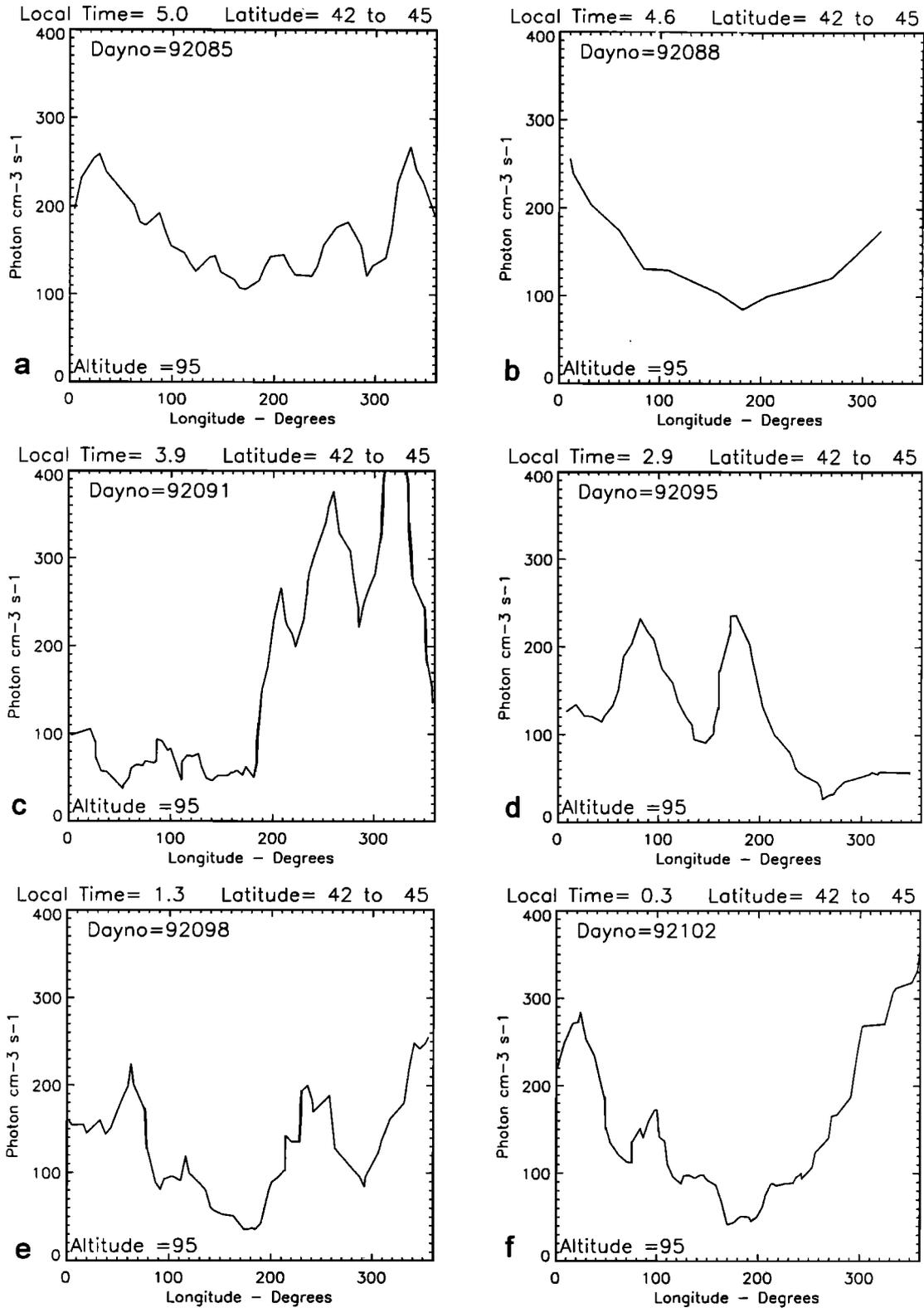
**Figure 8.** Volume emission rate (photons per  $\text{cm}^{-3} \text{s}^{-1}$ ) for the OI-558 nm emission at an altitude of 95 km plotted versus longitude for a latitude band  $40^{\circ}$ - $45^{\circ}$ N for six days during the northern springtime transition of March 25 to April 14, 1992, including (a) March 25, (b) March 28, (c) March 31, (d) April 4, (e) April 7, and (f) April 14.
