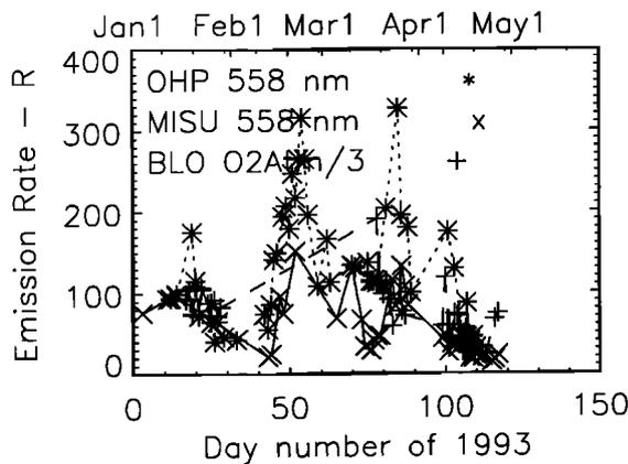
**Figure 1.** Vertically integrated (zenithal) emission rates for nighttime oxygen airglow for January-May, 1993, as observed at Observatoire de Haute-Provence (OHP), Meteorological Institute of Stockholm University (MISU), and Bear Lake Observatory (BLO) of Utah State University.
