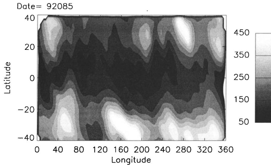
**Figure 5a.** Vertically integrated (zenithal) emission rate for the  $O(^1S)$  558-nm airglow measured by the wind imaging interferometer (WINDII) for March 25, 1992. The bar indicates the emission rate in rayleigh.
