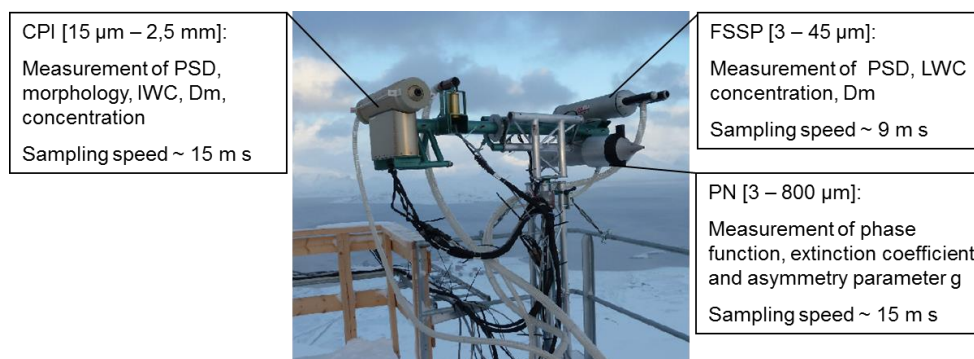
199 Figure 2: Cloud instrumentation used during CLIMSLIP. Indicated are: particle size range, 200 main cloud properties measured and theoretical sampling speed.
