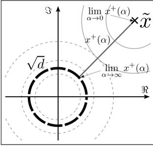
**Fig. 1.** Trajectory of  $x^+(\alpha) = \text{prox}_{\alpha f}(\tilde{x})$  as a function of  $\alpha$ .  $x^+(\alpha)$  follows the line where the level set of  $f$  (thin dashed circles) and  $|x - \tilde{x}|^2$  (thin circles) are tangent.
