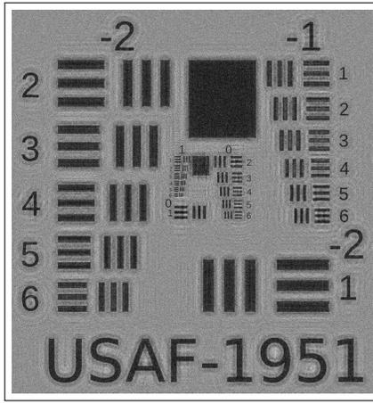
Fig. 7. Intensity of the estimated wave using the proposed proximity operator (noise standard deviation  $\sigma = 0.3$ ) back-propagated from  $z_A$  to  $z_0$ .  $\text{SNR}(x^+) = 7.60$  dB.
