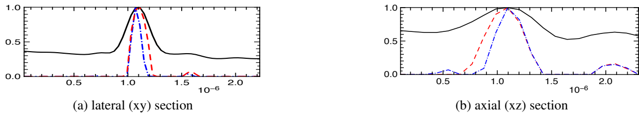
Fig. 2. Lateral and axial profile of the microtubule indicated by the green line on Figure 1.a for the wide field data (solid line), its blind deconvolution (dashed red), and the SIM (mixed blue).
