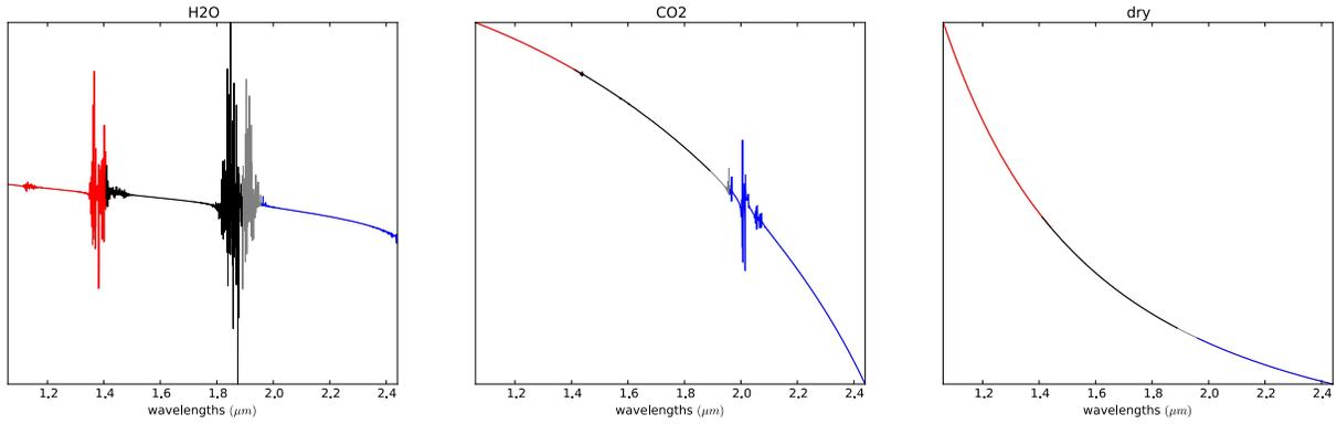
Figure 2. Example of components (H<sub>2</sub>O, CO<sub>2</sub>, dry) of atmospheric perturbation model as a function of the wavelength: Band J (red), H (black) and K (blue)
