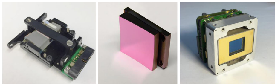
Fig. 7 Key elements of the ACS-NIR: (a) AOTF unit; (b) spectrometer autocollimating mirror; (c) InGaAs detector unit
