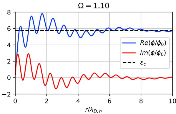
**Figure 6.** Real and imaginary parts of the electric potential  $\phi/\phi_0$  (blue and red lines, respectively) radiated at frequency  $\Omega=1.10$  in a two-electron temperature plasma  $\mu=0.11$  and  $\tau=100$ , together with  $\epsilon_c$  the asymptotic analytical limit of  $\text{Re}(\phi/\phi_0)$  (dashed line).
