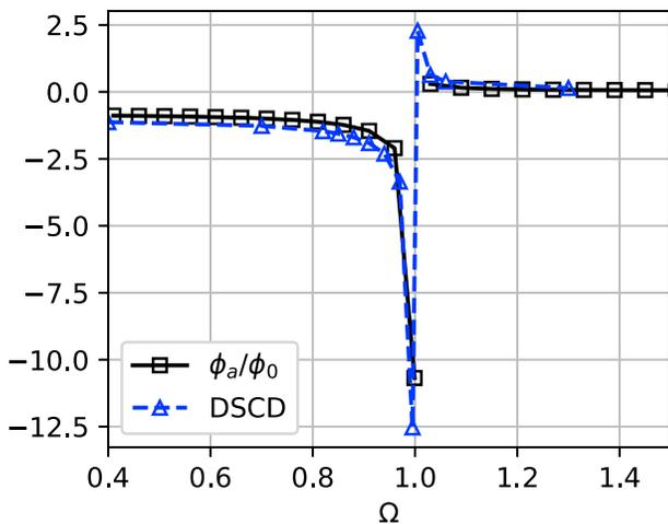
Figure 11. Amplitude of the radiated electric potential spectrum, expressed in logarithmic scale as  $20 \log_{10}(|\phi/\phi_0(\Omega, a/\lambda_D)|)$ , for  $a = 0.03$  m and  $\lambda_D = 0.3$  m, computed by equation (24) (squared black line) and by the Discrete Surface Charge Distribution (blue line).
