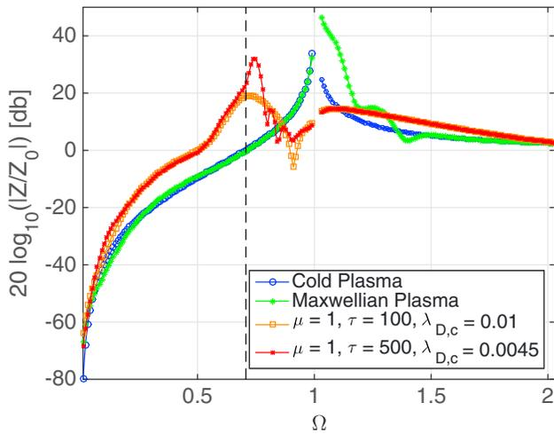
**Figure 8.** Normalized responses in power on the idealized mutual impedance probe (Figure 3) for different parameters  $\mu$  and  $\tau$ : cold electrons (blue), Maxwellian electrons (green), and a sum of two Maxwellian electrons configurations:  $\mu = 1$ ,  $\tau = 100$  (orange) and  $\mu = 1$ ,  $\tau = 500$  (red).
