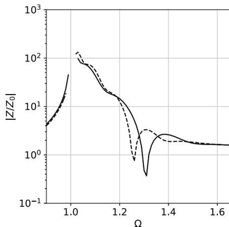
**Figure 7.** Normalized response, expressed in logarithmic scale as  $20 \log_{10} (|Z(\Omega)/Z_0|)$  for the Maxwellian case with  $\lambda_D=0.01$  m in black line on the double-dipole considered by Pottelette and Storey (1981) and for a sum of two Maxwellian evdf with  $\mu=0.01$ ,  $\tau=100$  and  $\lambda_{D,h}=0.70$  m in black dashed line.
