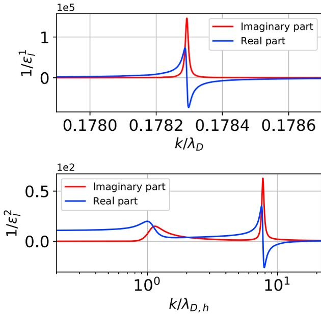
**Figure 1.** Real and imaginary parts of the (top) inverse of the dielectric function on the Maxwellian limit for  $\Omega=1.05$  and a (bottom) sum of two Maxwellian evdf for  $\Omega=1.05$ ,  $\mu=0.11$ , and  $\tau=100$  with a zoom on the neighborhood of the poles.
