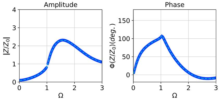
**Figure 4.** (left) Normalized response in modulus and (right) normalized response in phase for  $\lambda_D = 0.1$  m on the idealized mutual impedance probe geometry (Figure 3) considered by Beghin (1995).
