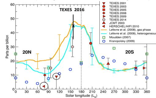
**Figure 3:** Seasonal variations of  $H_2O_2$  on Mars (observations and models), for a mean latitude of  $20N$  for  $L_s = 0-180^\circ$ , and  $20S$  for  $L_s = 180-360^\circ$ . The figure is adapted from [7].
