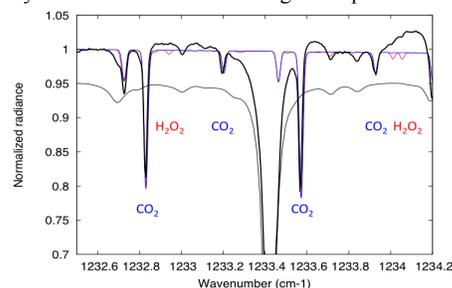
**Figure 1:** The disk-integrated TEXES spectrum between 1232.5 and 1234.2 cm<sup>-1</sup> (rest frequencies, thick black line). Models: CO<sub>2</sub> (blue), H<sub>2</sub>O<sub>2</sub> with a mixing ratio of 60 ppbv (red). Thin black line: standard atmospheric opacity at Maunakea Observatory, shifted vertically by 0.01 for clarity.
