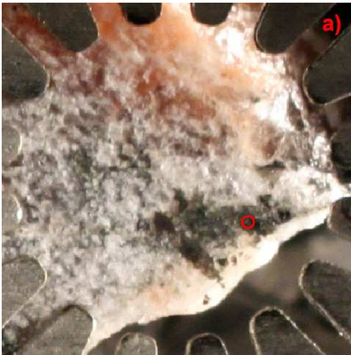
Figure A.2. ÄD sample for XPS after contacting with Tc(VII)-containing ÄGWS. Red circle indicates the region where Tc(IV) was found.
