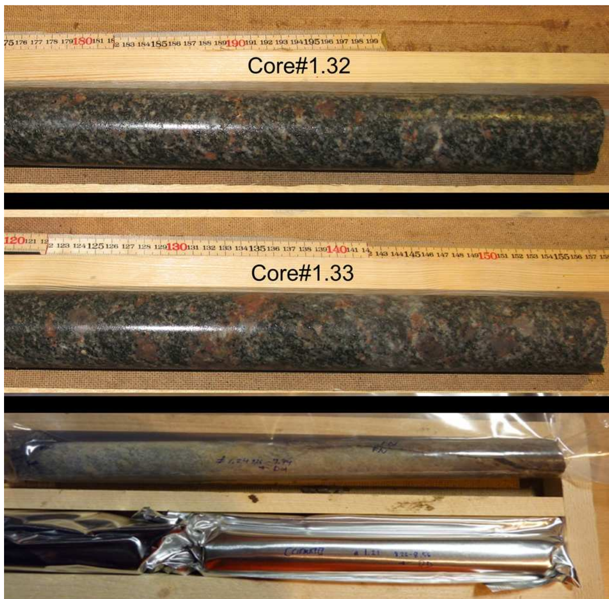
Figure A.1. (Top and middle) Cores used in the batch experiments directly after drilling. (Bottom) Two-layers packing of the cores, sealed into LD-PE and Al bags.
