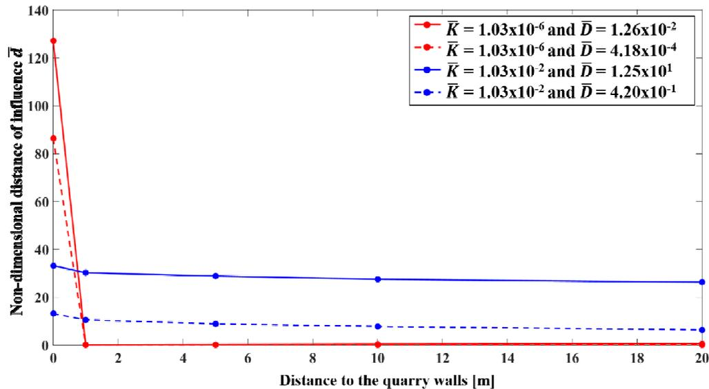
**Figure 5.** Non-dimensional distance of influence in a fracture located at a specific distance from the quarry walls. The aperture of the fracture is equal to  $4 \times 10^{-3}$  m. Different cases of rock matrix hydraulic properties are considered.
