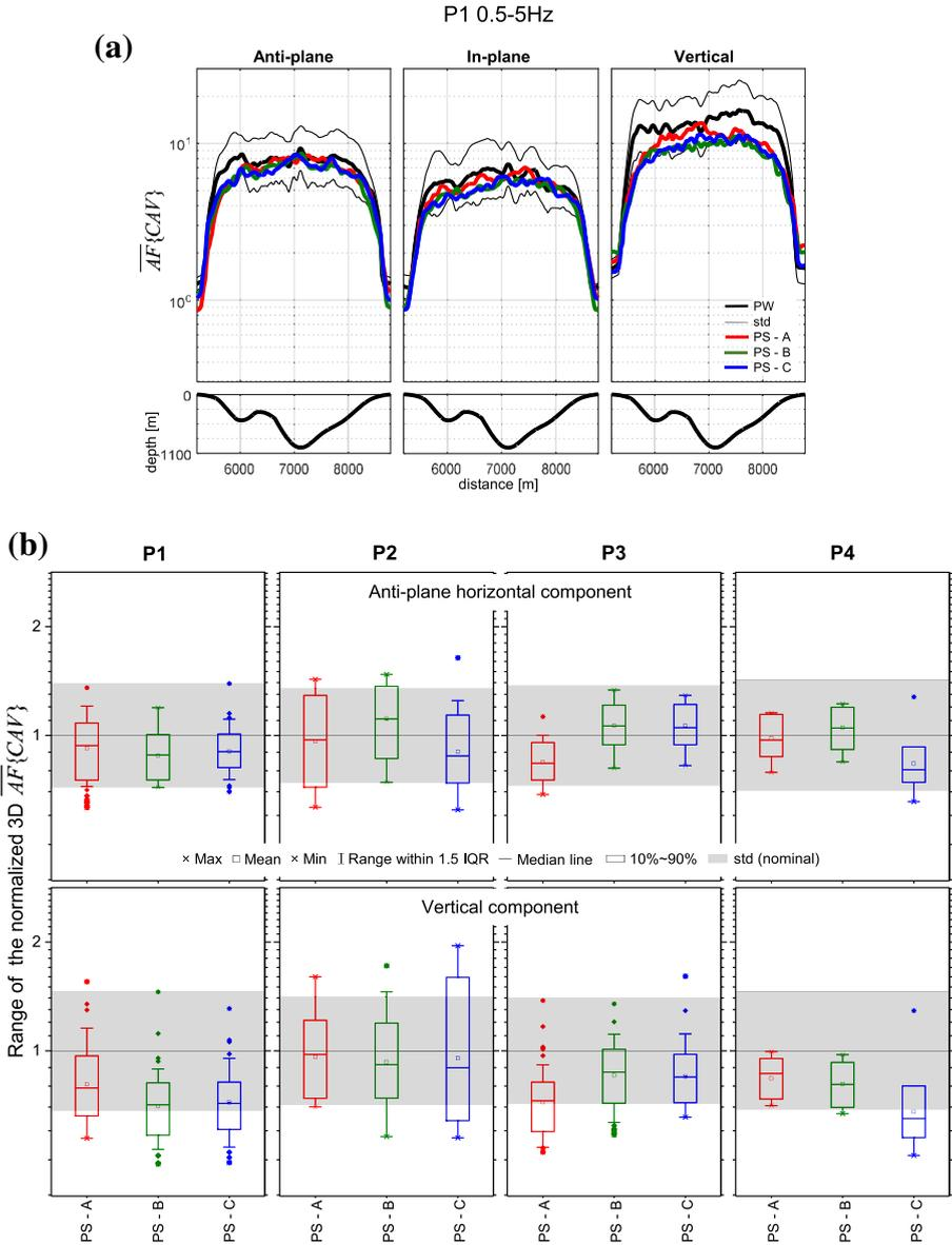
**Fig. 21** **a** Comparison of the amplification factors for CAV for 3 DC point sources A, B and C (PS—A, PS—B and PS—C), and plane wave excitation (PW) for profile P1 at Site 2 (Grenoble valley). **b** The range of amplification factor for CAV corresponding to the DC point sources A, B and C normalized by the amplification factor corresponding to the plane-wave excitation for the four profiles at Site 2 (Grenoble valley). The standard deviation represents the variability of the input motion
