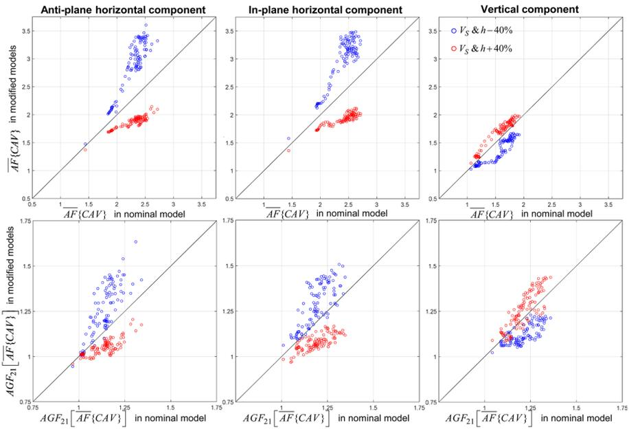
**Fig. 18** Comparison of the 2D amplification for CAV and 2D/1D aggravation factors for  $\overline{AF}\{CAV\}$  in the modified and nominal models of Sites 6 illustrating the effect of the simultaneous variations in the velocity and thickness of sediments with a fixed value of the local 1D fundamental resonant frequency
