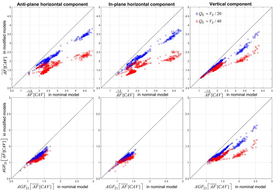
**Fig. 17** Comparison of the 2D amplification for CAV and 2D/1D aggravation factors for  $\overline{AF}\{CAV\}$  in the modified and nominal models of Sites 5–7 illustrating the effect of level of attenuation. Note that one symbol (empty circle) is used for all receiver positions at all sites
