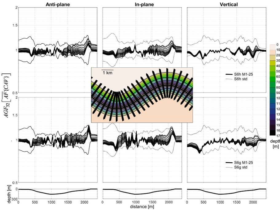
**Fig. 20** 3D/2D aggravation factors for  $\overline{AF}\{CAV\}$  for 25 profiles in the 3D model of the meander-like extension of 2D models S6h and S6g. The standard deviation represents the variability of the input motion
