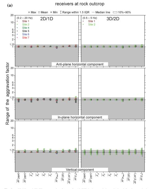
**Fig. 9 a** 2D/1D and 3D/2D aggravation factors for 10 EGM characteristics calculated for the nominal models. Each point represents a value at one receiver position at rock outcrop. *IQR* interquartile range. **b** The same as (**a**) but for receiver positions atop sediments. Excluded are receiver positions in case of the local fundamental frequency larger than 20 Hz
