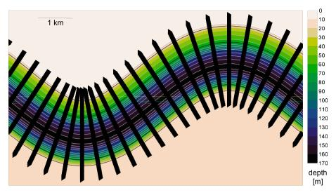
**Fig. 3** Depth of the sediment-bedrock interface in the 3D meander extension of 2D models of Site 6. Grenoble valley model (Site 2). Black lines indicate profiles of receiver positions
