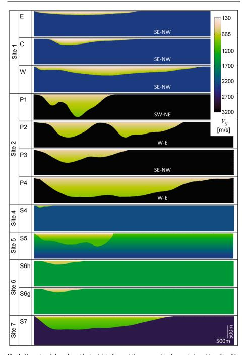
**Fig. 4** Geometry of the sediment-bedrock interface and S-wave speed in the nominal-model profiles. The profiles are denoted by symbols in the left column. The horizontal-to-vertical scale is 1:1. The S-wave speed is shown using colour scale by Niccoli (2014). *N* North, *S* South, *W* West, *E* East
