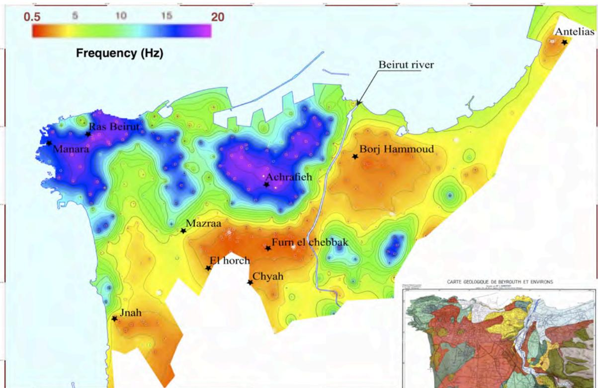
Figure 5. Map of the interpolated fundamental frequencies in the region of Beirut. Frequency is given in Hz. Bottom right : the geological map of the studied area
