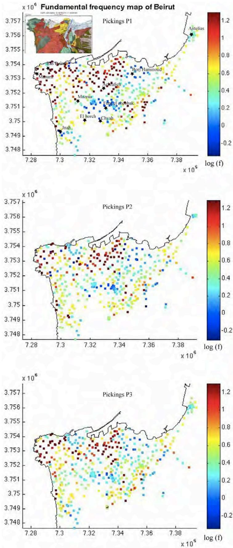
Figure 7. Comparison of the fundamental frequencies obtained by three independent pickings (P1, P2 and P3) of the H/V peaks. The color code on the right stands for the  $\log_{10}$  of the H/V peak frequency
