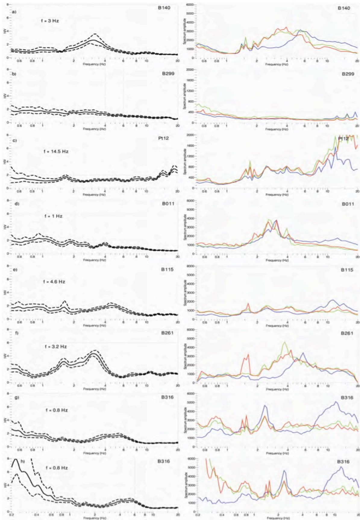
Figure 3. Examples of curves obtained in the analysis of the ambient noise measurements : (Left) H/V spectral ratios (mean  $\pm$  standard deviations) and (right) their corresponding Fourier spectra (blue: Z component, green: N/S component and red: E/W component). 3a : clear peak; 3b : flat curve on rock site; 3c : HF peak on rock site; 3d : flat curve on sediment site; 3e and 3f : sites with industrial peaks; 3g and 3h : high amplitudes at LF (<1 Hz)
