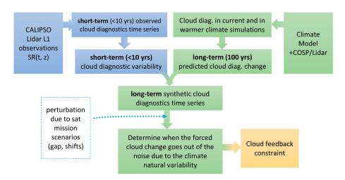
**Diagram 1.** Observation and model data processing chain. Lidar observation processing is in blue and illustrated in Figure 1. Processing of model output is in green. Cloud feedback constraints are in orange.
