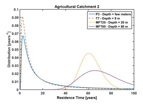
**Figure 6**: Illustration of the calibrated Inverse Gaussian RTD obtained on the agricultural catchment 2 (Saint Brice). The wells lying in the shallowest part of the aquifers have small residence times and exponential shapes. The wells lying in the deepest part of the aquifer display some skewed distributions.
