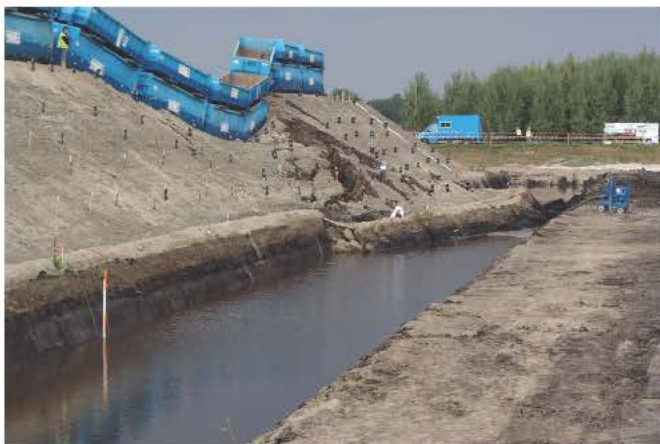
Fig. 3. Example of a physical model of a river dike taking a 1:1 approach ( http://www.dijkmonitoring.nl/en/projects/ ).
