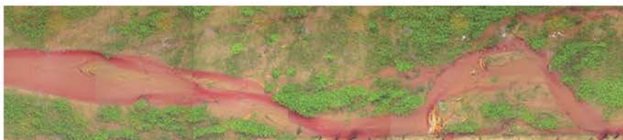
Fig. 7. Example of a physical model in which the original fluvial braided plain has been colonised by small-scale alfalfa vegetation. Flow is from right to left and the panel is 6 m long and 2 m wide.
