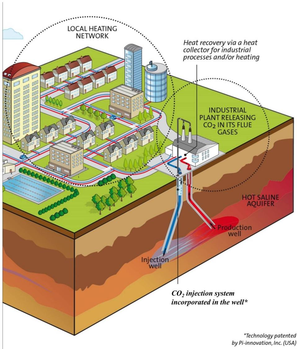
Figure 2 : Schematic view of the CO<sub>2</sub>-DISSOLVED concept [4]
