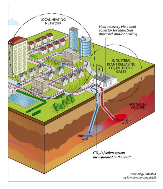
Figure 2 : Schematic view of the CO2-DISSOLVED concept [4]
