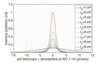
**Fig. 2.** Impulse response of the instrument–atmosphere system at 607.1 nm for several values of the Fried parameter  $(r_0)$ . The instrument parameters used are the focal of the SODISM II instrument  $(f_1)$  of 2.626 m, a pixel size of 13.5  $\mu$ m, and a pupil diameter  $(D_1)$  of 9 cm.
