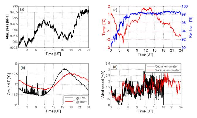
**Figure 4.** (a) Example of an unphysical jump in instantaneous values of pressure and (b) temperature in ground at 5 cm (black) and at 10 cm (red). (d) Example of unphysical persistence of high wind speed measurements using a cup anemometer due to frost in (c) (negative temperature in red and high humidity values in blue).
