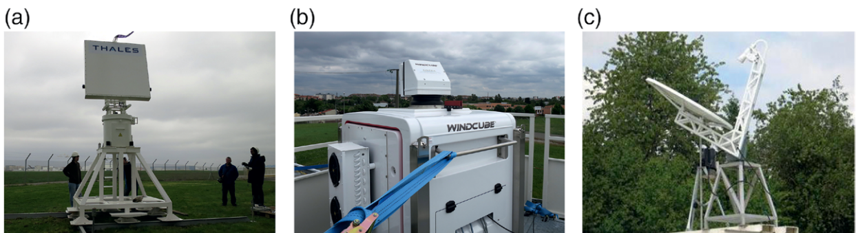
FIG. 1. Measurement systems in the UFO project: (a) the X-band Thales scanning radar, (b) the Leosphere scanning lidar, and (c) the X-band CURIE profiling radar.
