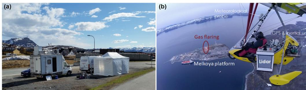
**Figure 2.** (a) Mobile atmospheric station (MAS) located near the Hammerfest Airport, equipped with the WALI Raman lidar. (b)  $N_2$  Raman lidar LAASURS embedded on a ULA. The ULA is flying over the Melkøya platform where a gas flaring is active.
