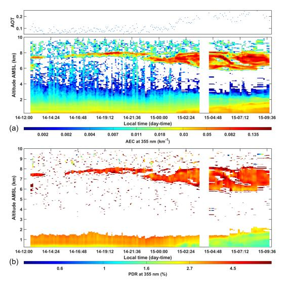
**Figure 5.** Temporal evolutions of (**a**) the lidar-derived aerosol extinction coefficient (AEC) and the aerosol optical thickness (AOT); (**b**) the particle depolarization ratio (PDR), at the wavelength of 355 nm, from 14 to 15 May 2016.
