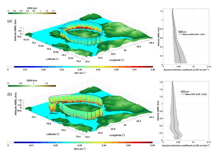
**Figure 9.** Vertical profiles of the aerosol extinction coefficient (AEC) derived from the lidar onboard the ULA: (a) flight 10 and (b) flight 11. The mean AEC vertical profiles and their dispersions are given in the graphs on the right. As in Fig. 4, the flights are plotted over the digital elevation model (DEM) GTOPO30.
