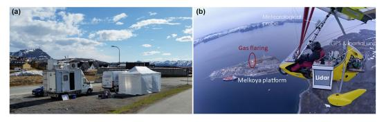
**Figure 2.** (a) Mobile atmospheric station (MAS) located near the Hammerfest Airport, equipped with the WALI Raman lidar. (b)  $N_2$  Raman lidar LAASURS embedded on a ULA. The ULA is flying over the Melkøya platform where a gas flaring is active.
