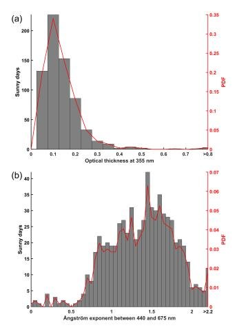
**Figure 18.** Histograms of (a) the aerosol optical thickness at 355 nm and (b) the Ångström exponent between 440 and 675 nm for the AERONET station of Andenes ( $69^{\circ}$  N,  $16^{\circ}$  E). The data are for the clear days between 2008 and 2016. The probability density functions (PDFs) are also given.
