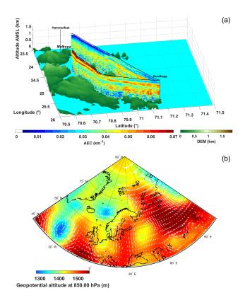
**Figure 11. (a)** Vertical profiles of the aerosol extinction coefficient (AEC) derived from the lidar onboard the ULA for flight 13 on 22 May, 21:38-23:58 UTC. As in Fig. 4, the flights are plotted over the digital elevation model (DEM) GTOPO30. (b) Geopotential altitude for the pressure level of 850 hPa ( $\sim 1.6$  km a.m.s.l.) at 00:00 UTC on 23 May 2016. The wind field at 850 hPa is also indicated in white arrows.
