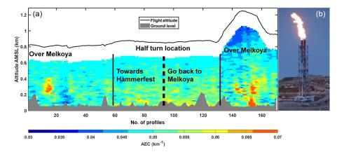
**Figure 10. (a)** Vertical profile of the aerosol extinction coefficient (AEC) during flight 4 (16 May, 22:39–23:24 LT) dedicated to the sampling of the Melkøya flare at 355 nm. (b) Flare sampled by the airborne lidar over the Melkøya platform.
