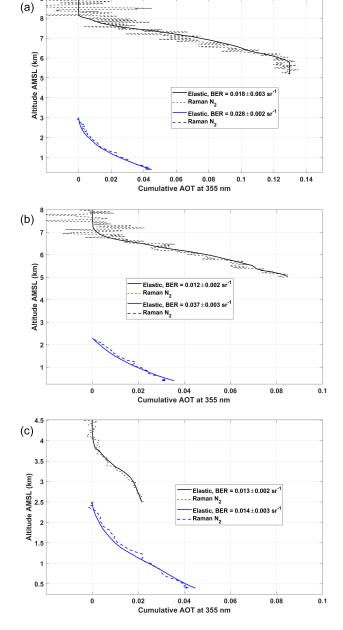
**Figure 8.** Cumulative aerosol optical thickness (AOT) derived from both the  $N_2$  Raman (dashed line) and the elastic (continuous lines) channels for the upper (black lines) and the lower (blue line) aerosol layers at 355 nm: (a) 14–15 May, (b) 20–21 May, and (c) 22– 23 May.
