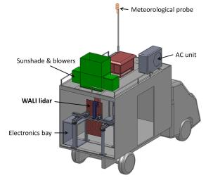
Figure 3. Schematic representation of the MAS equipped with the Raman lidar WALI.
