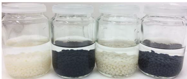
Figure 2. Photograph of pure and hybrid hydrogel CS beads. The mean diameter of the beads was 2 mm.
