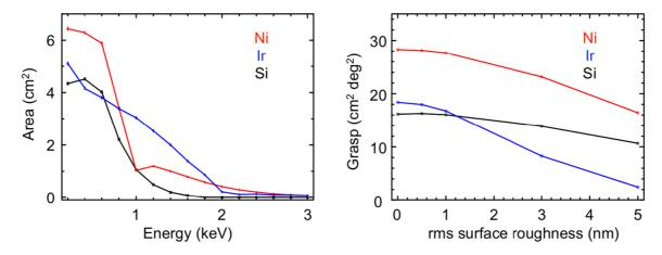
**Fig. 48** *Left Panel*: The on-axis effective area per optic of a 4 inch optic with focal length of 25 cm as a function of energy. Different colors correspond to different coatings. Mirror surface roughness is fixed at 1 nm rms. *Right Panel*: The grasp at 600 eV as a function of the mirror surface roughness in rms (Mitsuishi et al. 2016)
