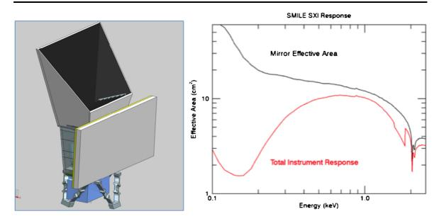
**Fig. 56** *Left Panel*: CAD model of SXI showing baffle (top) main telescope tube (center) and front-end electronics box (bottom) with the radiator panel in front. The data processing unit and power supply box are not shown. *Right Panel*: Instrument response showing the mirror effective area (black) and total response including CCD QE and optical filter transmission (red)
