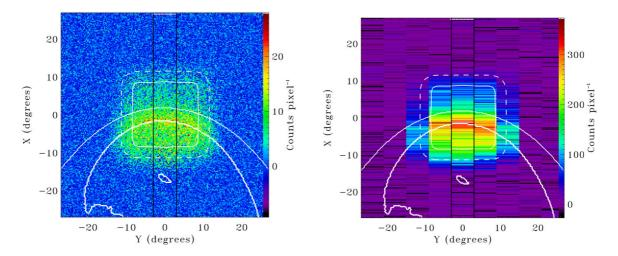
**Fig. 60** Left Panel: Simulated image drawn from the model image from Fig. 57 with the addition of backgrounds, convolution with the point spread function, and multiplication by the vignetting function, and the addition of instrumental noise. Right Panel: the simulated image rebinned to preserve the high resolution perpendicular to the magnetopause but maintain high signal-to-noise values in each pixel. The binned pixels are  $6^{\circ} \times 0.25^{\circ}$
