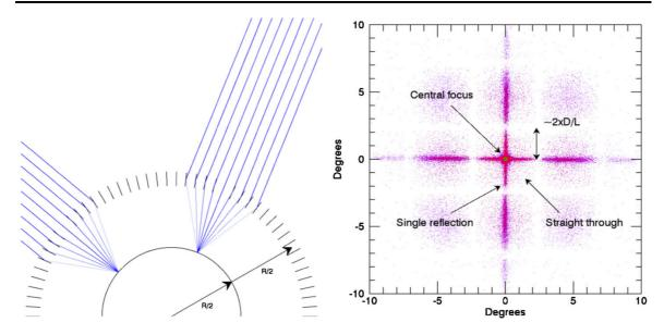
**Fig. 49** *Left Panel*: Simplified view of the focusing geometry for a Lobster-eye optic. X-rays that make grazing incidences on the optics are focused only a detector plane at half the radius of curvature. *Right Panel*: Binned image for a micropore optics point spread function generated by a ray-tracing simulation. The image has been logarithmically scaled to emphasize the structure at large off-axis angles. Labels indicate the origin of various features in the image
