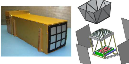
**Fig. 53** Left Panel: STORM prototype X-ray imager with a  $3 \times 3$  optics assembly at the front and an electronics assembly at the back (Collier et al. 2012). Right Panel: Complete module concept which has a  $10 \times 10$  micropore optics array and a  $3 \times 2$  MCP detector array. A baffle shields the optics from solar and terrestrial emissions
