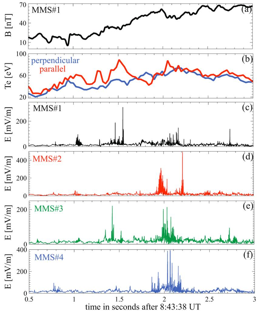
**Figure 1.** The bow shock crossing by MMS on 30 November 2015: (a) the magnetic field magnitude and (b) electron parallel and perpendicular temperatures measured aboard MMS#1; (c–f) magnitude of the electric fields measured at four MMS spacecraft. MMS = Magnetospheric Multiscale Mission.
