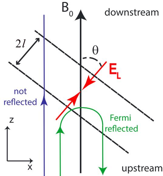
**Figure 3.** The schematics of approximately 1-D planar electrostatic solitary waves with a convergent electric field configuration:  $E_L$  is the dominant bipolar electric field,  $2l$  is the typical spatial width, and  $\theta$  is the electric field inclination angle to the local DC magnetic field  $\mathbf{B}_0$ . Thermal electrons streaming from the upstream (downstream) region can be either Fermi reflected back to the upstream (downstream) region or pass through.
