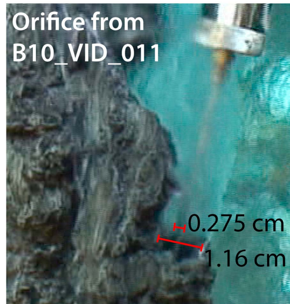
Figure 6. A cropped image of the vent orifice corresponding to video B10_VID_011. The diameter of the vent orifice (long, red line) is measured based upon the known width of the gas sampler in the image (short, red line). The measured radius (0.58 cm) compares closely with that calculated for B10_VID_011 (0.56 cm).
