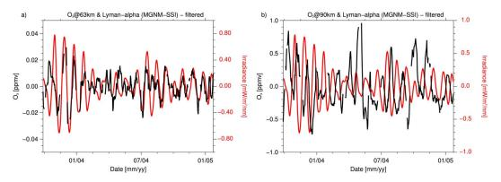
**Figure 4.** Temporal evolution of anomalies of (red) Lyman- $\alpha$  line and (black) ozone measured by GOMOS at (a) 63 km and (b) 90 km. The time series have been digitally filtered (see section 2.3 for details). SSI = solar spectral irradiance; GOMOS = Global Ozone Monitoring by Occultation of Stars.
