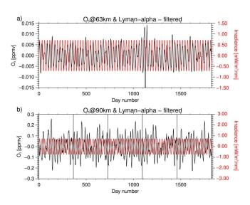
**Figure 5.** Temporal evolution of anomalies of (red) Lyman- $\alpha$  line and (black) ozone simulated by periodically forced HAMMONIA experiment at (a) 63-km and (b) 90-km altitudes. The time series have been digitally filtered. HAMMONIA = Hamburg model of the neutral and ionized atmosphere.
