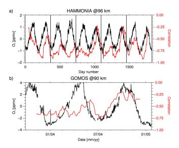
**Figure 9.** Temporal evolution of the unfiltered ozone anomalies (in black) and of the sliding correlation coefficients (in red, see text for details) between the filtered ozone and the Lyman- $\alpha$  line time series for (a) the model at 96 km and (b) the observations at 90 km. GOMOS = Global Ozone Monitoring by Occultation of Stars; HAMMONIA = Hamburg model of the neutral and ionized atmosphere.
