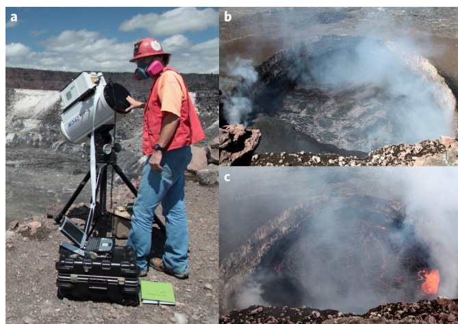
Fig. 1 | Instrument set up and lava lake behaviour at Halema'uma'u on 5 March 2013. a , Fourier transform infrared spectrometer with telescope pointed at the lava lake some 200 m distant. b , Initial regime of mild degassing (non-spattering). c , Subsequent regime of vigorous degassing (spattering). The lava lake is approximately 200 m across.
