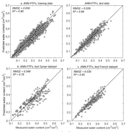
670 671 672 673 Figure 7: Measured and predicted water content (cm<sup>3</sup>/cm<sup>3</sup>) recorded with the artificial neural networks using soil properties (clay, silt, sand, organic carbon and bulk density) for the French national database (Al Majou et al., 2008b) (a), Syrian dataset (b) and the French dataset (c).
