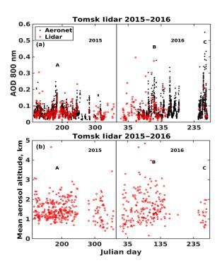
**Figure 8.** Time evolution from April 2015 to September 2016 of the 808 nm AOD for lidar (red) and sun-photometer (black) observations (**a**) and corresponding aerosol altitudes  $z_{aer}$  given by Eq. (2) (**b**). A, B, and C are the cases analysed in Sect. 5.
