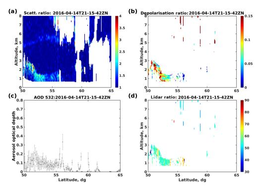
**Figure 14.** Latitudinal cross section of CALIOP 532 nm scattering ratio  $R_{532}$  (**a**), aerosol depolarization ratio  $\delta_{532}$  (**b**), aerosol optical depth AOD<sub>532</sub> (**c**) and lidar ratio  $S_{532}$  (**d**) for 14 April 2016.
