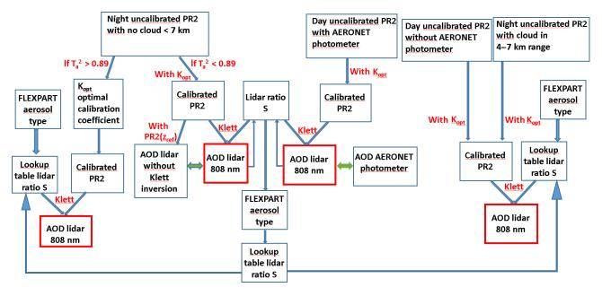
**Figure 4.** Flow chart of the lidar range-corrected signal (PR2) processing to derive the 800 nm aerosol optical depth (AOD) up to the reference altitude ( $z_{ref}$ ). Four different calibrations and AOD calculations are used according to the measurement conditions. Iteration between the AOD calculation and the lidar ratio value is only possible when the AOD is compared to an external AOD reference (green two-sided arrows).
