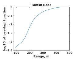
**Figure 2.** Geometrical overlap function used for the correction of the lidar data in log10 scale between 100 and 500 m.
