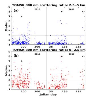
**Figure 7.** Time evolution from April 2015 to September 2016 of the median of the 808 nm Tomsk lidar backscatter ratio for two altitude ranges: 0–2.5 km (**b**) and 2.5–5 km (**a**). A, B and C are the cases analysed in Sect. 5.
