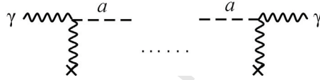
Figure 4.11.2: Left: \gamma \rightarrow a conversion in the external magnetic field \mathbf{B} (in stars the rôle of \mathbf{E} and \mathbf{B} is interchanged). Right: inverse process a \rightarrow \gamma .
