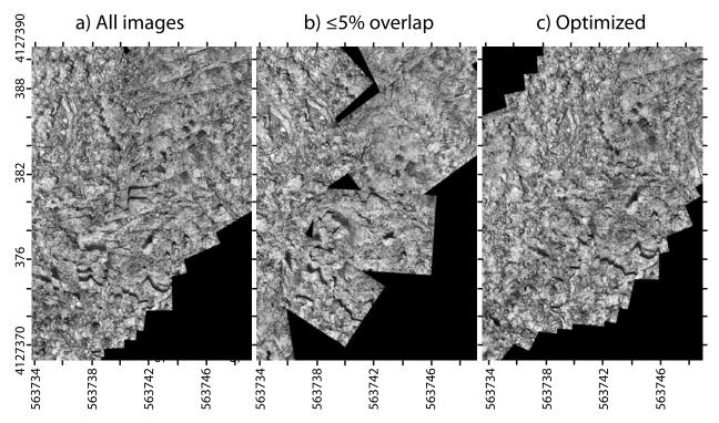
**Figure 6.** Comparison of three mosaics from an area of the Lucky Strike Field. (a) The mosaic including all images shows areas with overlapping frames that hinder the visualization of the terrain. (b) The mosaic with a reduced number of photos allows a clear view of individual frames and therefore of seafloor textures and structures, although with reduced coverage. (c) The optimized mosaic shows continuous imagery across frames, after correction of the navigation and reprojection of images.
