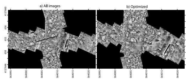
**Figure 7.** Along- and across-track errors in positioning, scaling and rotation of images in the (a) navigated and (b) optimized mosaics. Dashed lines indicate the same feature in different frames, and the solid black line shows both rotation and scaling differences across tracks. Errors in locations along-track are typically <2 m, while those across track are <10 m (dashed lines).
