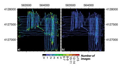
**Figure 3.** Map of the study area showing the overall image coverage and the number of images over a given area (see tracks in Figure 2). (a) The mosaic containing all the images shows areas with considerable image overlap near some of the vents and at turns. (b) Image repetition is considerably reduced if consecutive images with  $\leq 5\%$  overlap are retained. Two photomosaics are built with all the images in Figure 3a and the subset shown in Figure 3b (see text for details).
