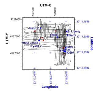
**Figure 2.** ARGO II tracks over the Lucky Strike hydrothermal field. Relief in the area reaches >100 m (10-m contours, derived from ARGO II depth and altimetry [Scheirer et al., 2000]). The main high-temperature vents are also indicated. UTM coordinates and reference system correspond to the transponder navigation deployed for the LUSTRE'96 cruise. Red boxes and associated numbering correspond to the location of panels in Figures 9 and 10.
