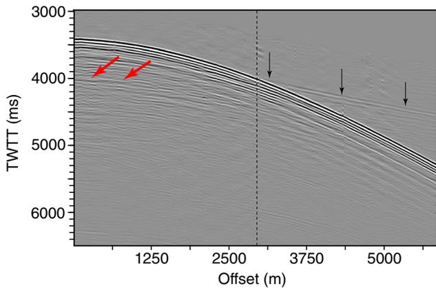
**Figure 3.** Shot gather extracted from the 2-D seismic line at  $\sim 9^{\circ}53'N$  after applying processing flow outlined in the text. Black arrows show first refraction event; dashed vertical line shows the offset at which the refraction event emerges ( $\sim 2,975$  m); red arrows mark the presence of the AML reflector.
