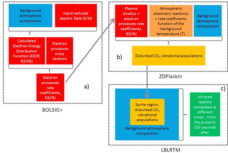
**Figure 1.** Computation pipeline for the simulation of the plasma kinetics of a sprite streamer and subsequent time-dependent thermal infrared radiative emissions. (a) Stands for the plasma parameters computation, (b) for the solving of the kinetic scheme, and (c) for the radiative transfer computations.
