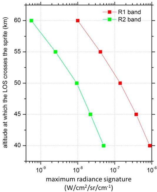
**Figure 7.** Maximum signature of a sprite as a function of the altitude at which the LOS crosses the sprite-disturbed region. The observer is located at 30 km of altitude, and the zenith angle of the LOS varies so that it crosses the sprite between 40 and 60 km of altitude. The distance is unchanged ( $d = 50$  km), and we kept a sprite diameter of 10 km. LOS = line of sight.
