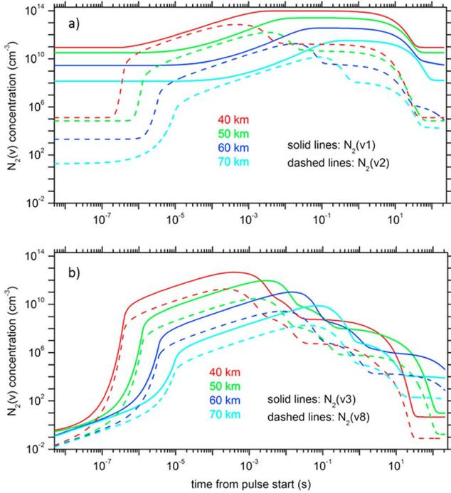
**Figure 3.** Time evolutions of the concentrations of  $N_2$  vibrational levels from 40 to 70 km of altitude. Panel (a) shows the concentrations of the first and second  $N_2$  vibrational levels. Panel (b) shows the concentrations of the third and eighth  $N_2$  vibrational levels.
