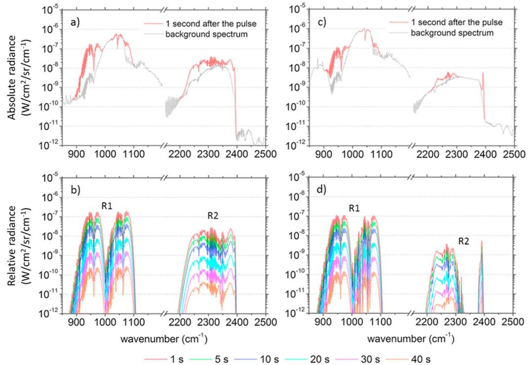
**Figure 5.** Absolute spectra of background atmosphere, in gray, and sprite, in red, for an observer located at 40 and 20 km of altitude, (a) and (c), respectively. Time evolution of the sprite signature (i.e., sprite spectra – background spectrum) for an observer located at 40 and 20 km of altitude, (b) and (d), respectively. The absolute sprite spectrum (red curve, graphs a and c) are computed 1 s after the pulse. Thus, it represents the maximum signal.
