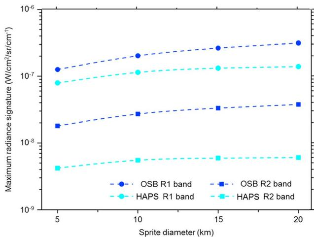
**Figure 6.** Maximum signature of a sprite as a function of its diameter for observers located in the stratosphere. The OSB and HAPS cases are represented in deep and light blue, respectively. The geometrical setup is the same as previously, likewise the time (1 s after the pulse) and the spectral resolution (1 cm<sup>-1</sup>). OSA = open stratospheric balloons; HAPS = high-altitude platform system.
