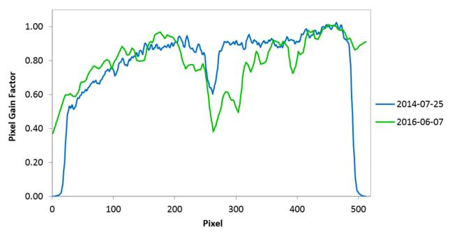
Fig. A.6. Pixel gain factors for each individual pixel on Row A for GS16. The 2014-07-25 and 2016-06-07 curves were measured early and late in the mission, respectively.
