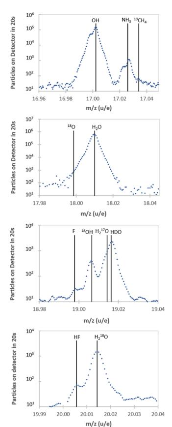
**Fig. A.2.** Sample DFMS mass spectra (from 2014-10-20) for m/z 17–20 u/e.
