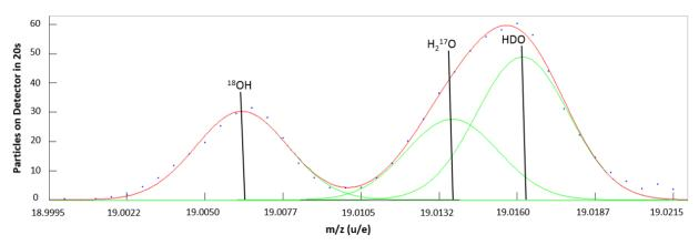
Fig. 4. Sample DFMS mass spectrum from 2016-03-03 T 03:45 illustrating the use of manual peak-fitting with equal-width Gaussians to separate the  $H_2^{17}O$  peak from that of HDO. Dotted line: mass spectrum, green lines: fitted Gaussians, red line: sum of fitted Gaussians.
