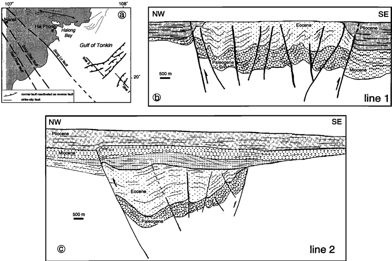
**Figure 4.** Location (a) and interpretation of two seismic lines (line 1 (b), line 2 (c)) in the Gulf of Tonkin, showing tectonic inversion of graben. Inversion occurred sometime after Pliocene unconformity.
