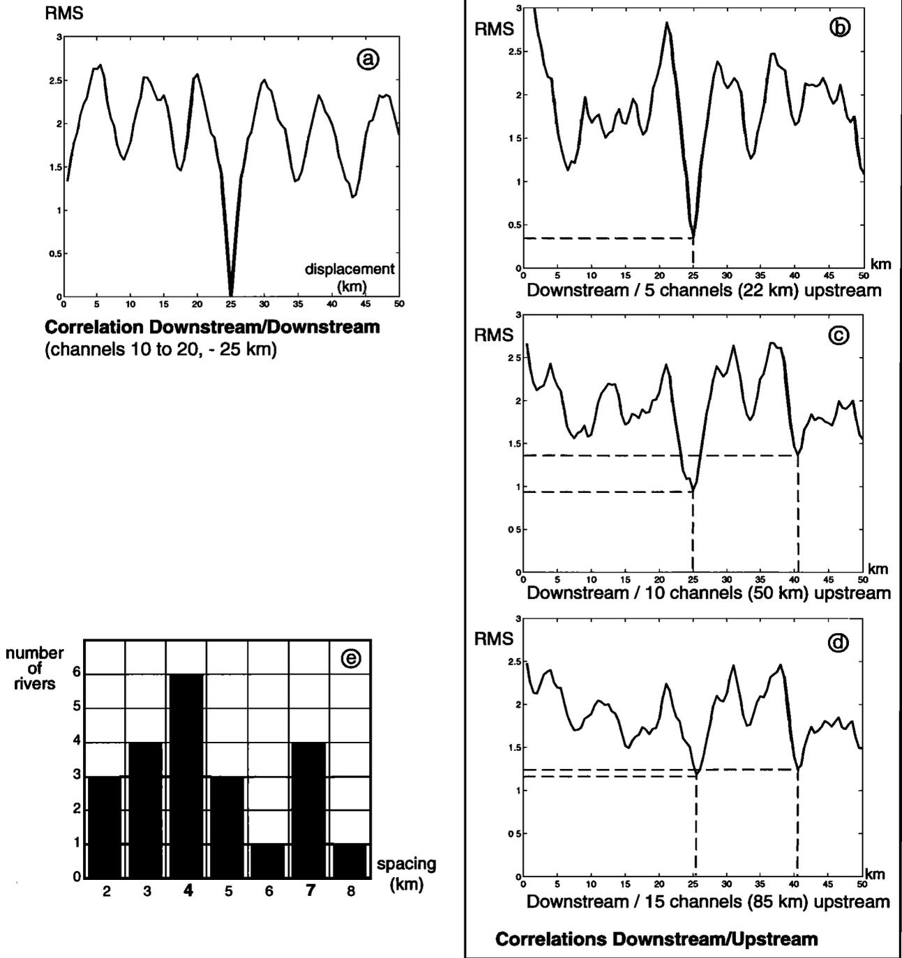
**Figure 8.** (a) Calibration test on artificial perturbation of drainage network obtained by offsetting, then correlating the downstream side with itself. (b) to (d) Correlation between downstream side and upstream side. Restored displacements along RRF versus root mean square (RMS) of distances between each upstream channel and closest downstream channel. (e) Histogram of spacing of upstream rivers showing main peak at 4 km and smaller one at 7 km.
