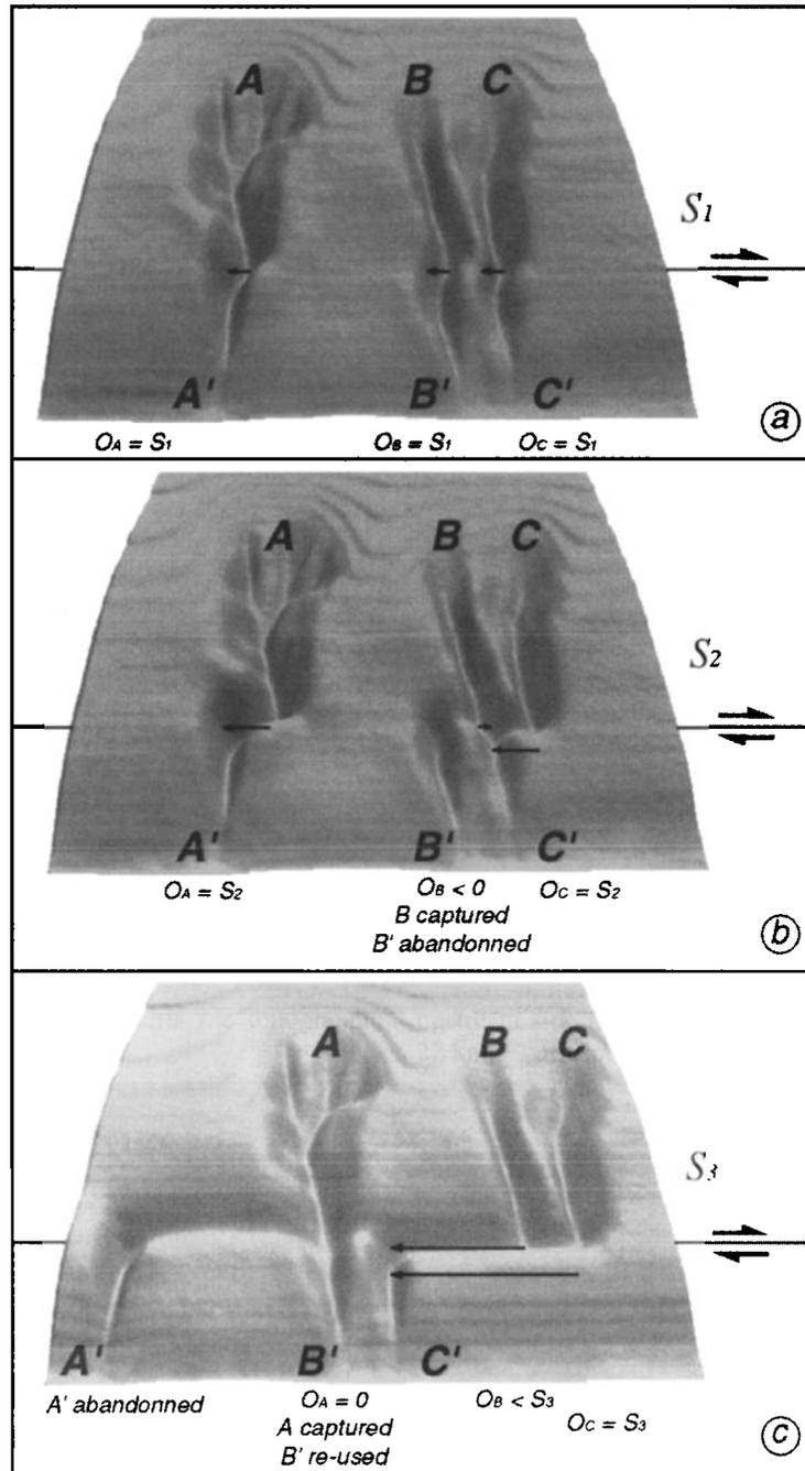
**Figure 6.** Sketches of 3-D drainage system perturbation by strike-slip fault with increasing fault displacement from (a) to (c). DEM is derived from a simplified topographic map. Successive stages are obtained by cutting and sliding initial map, restoring by hand continuity of topographic contours, and interpolating new contours to produce the next DEM. ( $O_x$ , offset of river channel X;  $S_i$ , slip along fault at stage  $i$ ). See discussion in text.
