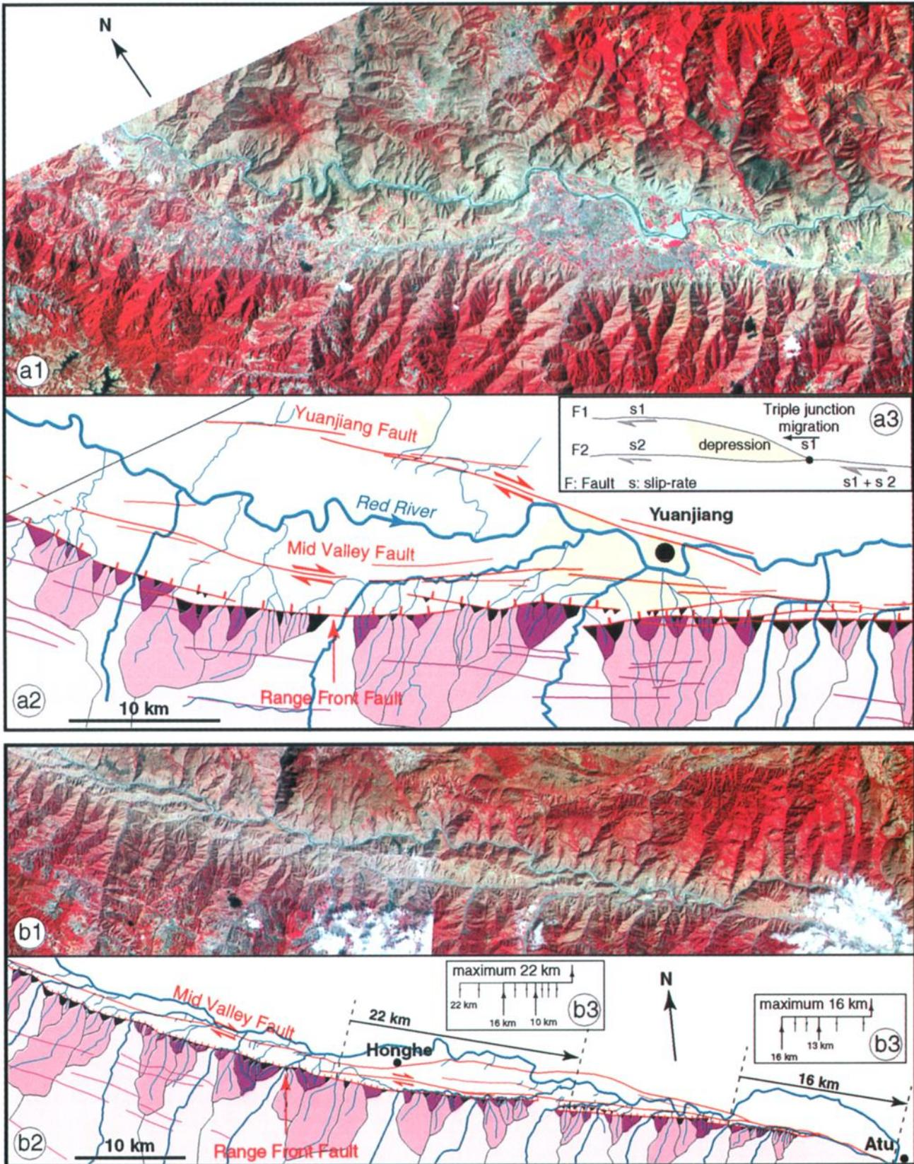
**Plate 2.** Same symbols as for Plate 1. (a) Yuanjiang stretch of the RRF. (a1) SPOT image (KJ 260-303). (a2) Corresponding map. (a3) Interpretation of the "junction" basin due to interaction and slip transfer between strike-slip fault stands at Yuanjiang. (b) Honghe-Atu stretch of the RRF. (b1) SPOT image mosaic (KJ 261-303 and 262-303). (b2) corresponding map. (b3) Largest offsets observed on Mid Valley fault, with their different significance.
