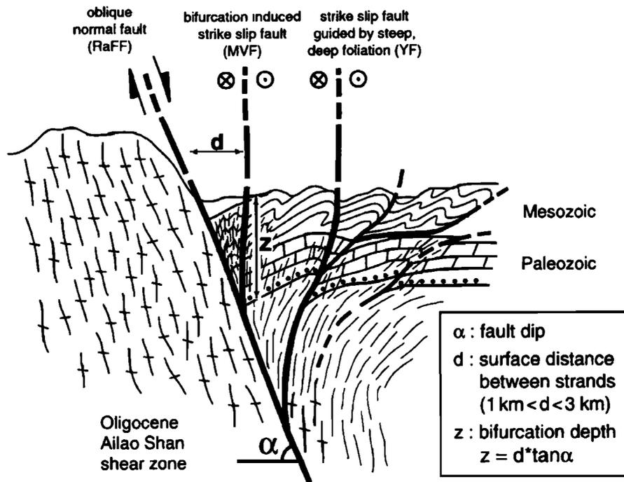
**Figure 10.** Schematic cross-section showing separation into normal and strike-slip strands for fault with oblique motion at depth [after Armijo *et al.*, 1986]. Bifurcation point can be at one sedimentary interface in cover (Mesozoic red sandstones or calcareous Paleozoic).
