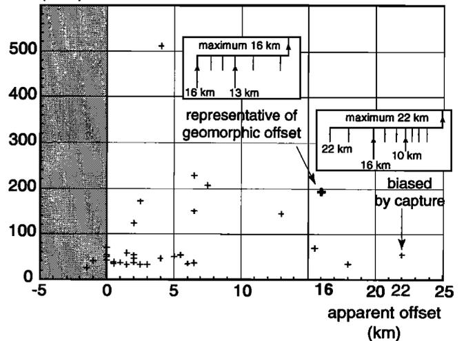
**Figure 5.** Plot of the drainage areas >15 km<sup>2</sup> as a function of apparent river offsets. Offsets are mostly right lateral (80% of 32 rivers). See text for discussion.
