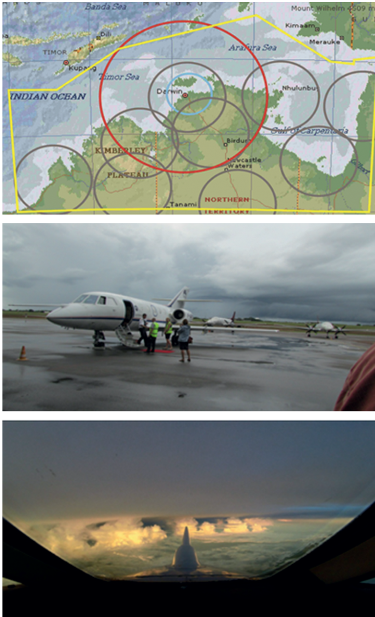
FIG. 4. (top) Operating area of the HAIC–HIWC Darwin flight campaign (yellow polygon) with ground-based radar coverage indicated by gray rings, including the research C-band polarimetric (CPOL) radar (blue ring). The red ring shows a 300-nmi-distance reference. (middle) The SAFIRE Falcon 20 aircraft prepares for a research flight. (bottom) Monsoon convection sampled within the Darwin operating area. Photos provided by T. Ratvasky.
