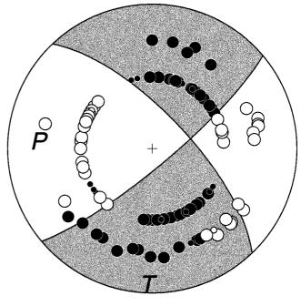
**Figure 4.** Focal mechanism of the main shock (lower-hemisphere Schmidt projection). Full symbols: compression; open symbols: dilatation; symbol size is smaller when first motion is emergent. Preferred fault plane strikes N136°E, with a 70°NE dip.
