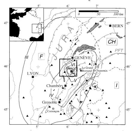
**Figure 1.** Area shaken by the 1996 July 15 Epagny earthquake. Isoseismal curves from the Bureau Central Seismologique Français. Triangles show permanent seismic stations. Chamonix, Corrençon and Le-Grand-Bornand are the sites of three damaging earthquakes discussed in the text. Principal Late Cenozoic thrusts are indicated. PFT=Penninic Frontal Thrust. Boxes show frames of Figs 2(b) and 3. Inset shows geographical location.
